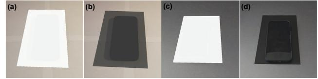
**Figure 3:** (a) shows a white hologram with a white surface, effectively concealing the phone. (b) shows a dark hologram on a white surface, where the phone remains translucent. (c) shows a white hologram on a dark surface, where the hologram becomes prominent. (d) shows a dark hologram on a dark surface, where translucency reveals the phone, demonstrating the limited effectiveness of darker holograms for concealment.
