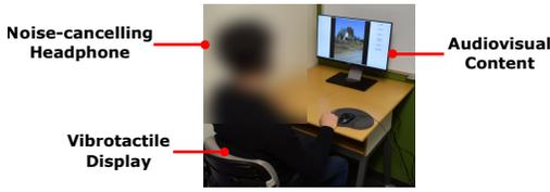
**Figure 6: Participants sat against a chair cushion with vibrotactile actuators during the study. The vibrotactile device provided tactile stimuli that were synchronized to the shown videos.**
